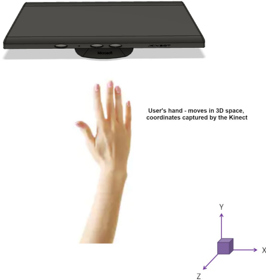
Figure 7. A visual of how the user will interact with the Kinect in a 3D space.
